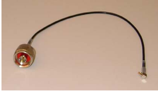
Figure 10: N-type to MC card adapter cable that is included with the J8448A ProCurve yagi antenna
